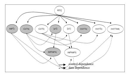
Figure 2: The PDG of the example program from Figure 1(a) and the grey vertices represent the slices of statement from Figure 1(b)
