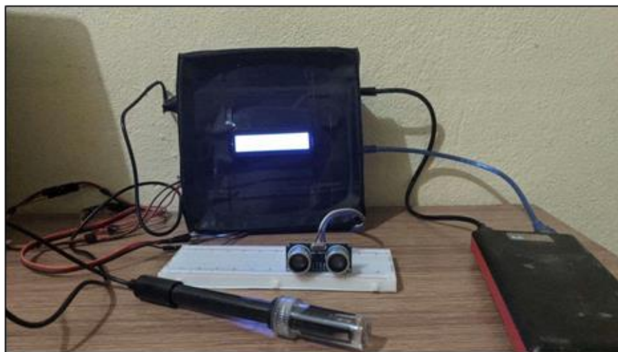
Figure 4: Prototype of Automated Alert System for River Water Level and Water Quality Assessment using Telegram Bot API
