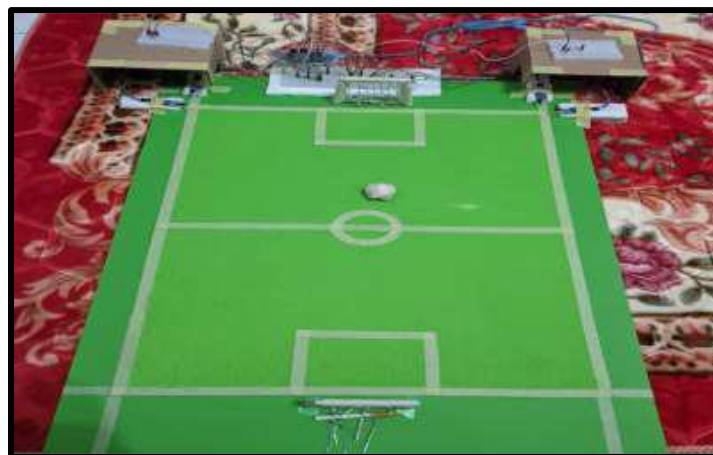
Figure 5. The prototype of a football pitch that combining the sensors.
