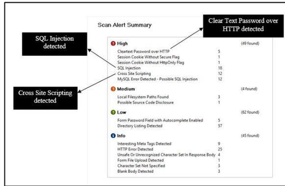
Figure 4 Result for scanning vulnerabilities
