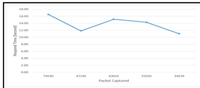
Figure 3 Response Time Graph with Dos Attack
